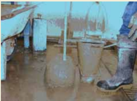
Slump test conducted during trial mix
