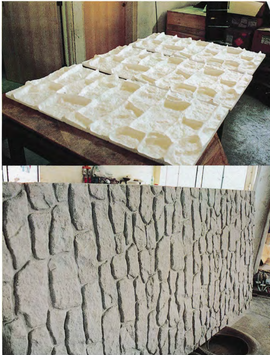
A stone-effect precast wall using polystyrene mould technique which has a range of surfaces to choose from and is available from local precasters
