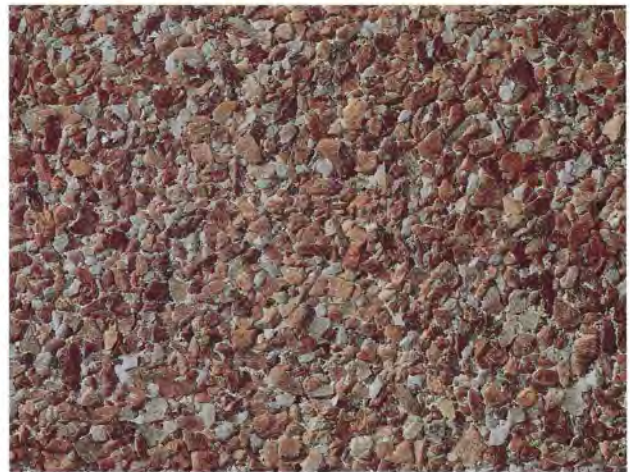
Coarse and fine aggregates of white marble, pink stones, white cement with a light retardant
