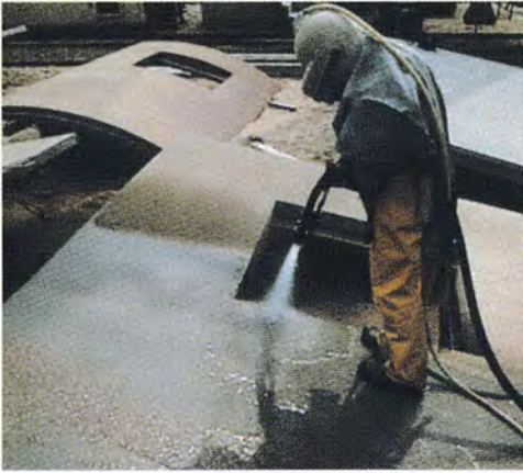
Sand blasting in factory-controlled environment
