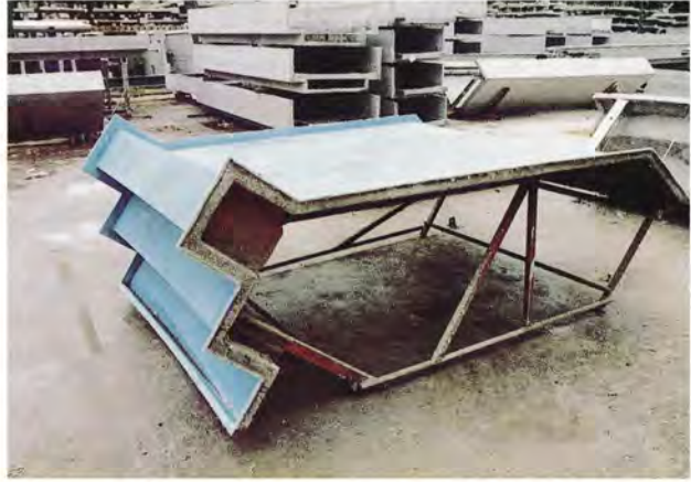
A GRC mould for a relatively complex corner feature for King's Centre Development Singapore
