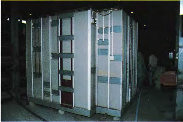
Pre-assembled bathroom cell prior to delivery
