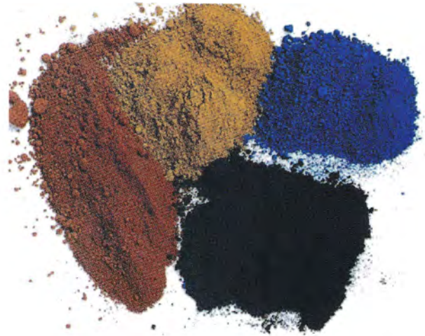
Coloured concrete are from metallic oxides. Iron oxide for black, oxide for blue red and yellow chromium for green cobalt Natural organic pigments are relatively cheap but colours are not consistent
