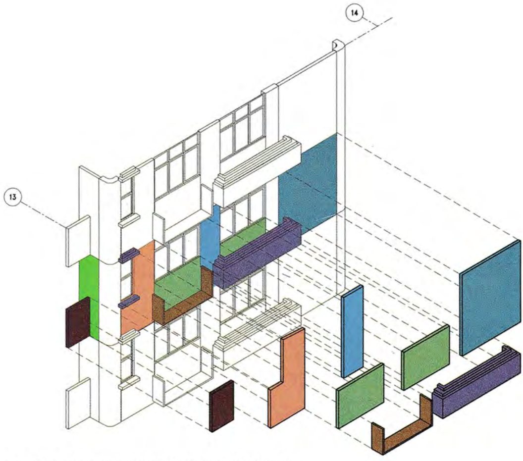
PROPOSED PRECAST CONCRETE PANELS: TYPE 'B'
