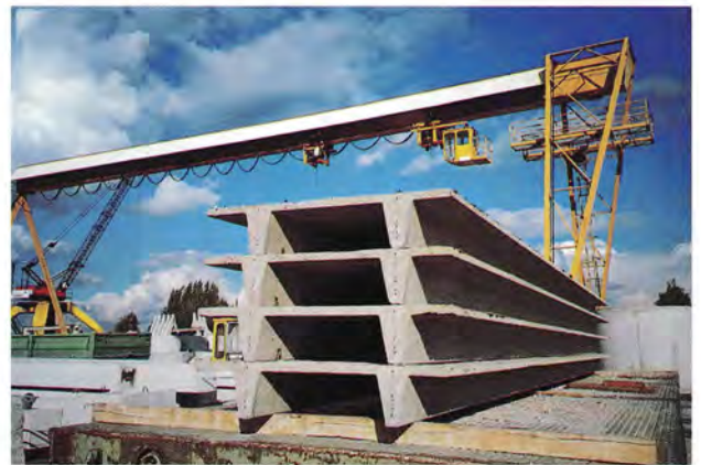
Double-T floors ready for delivery in a Belgium factory
