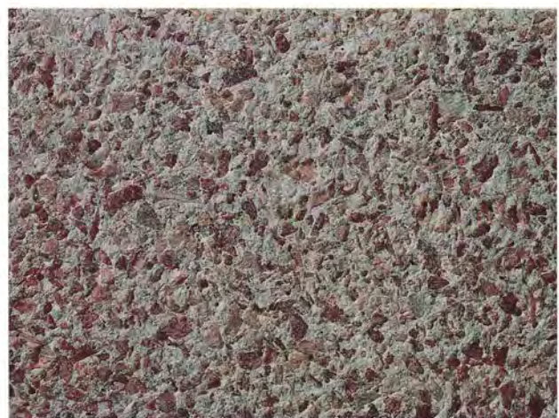
Similar constituents as above with a light acid etched finish. Chemical retarding agents are available to produce a range of retarding effects to provide light, medium or heavy surface expose levels
