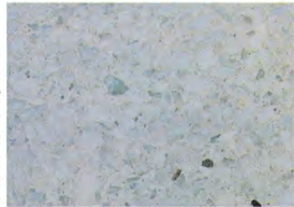
A machine polished finish Cement white Fine aggregate crushed white marble Coarse aggregate white marble
