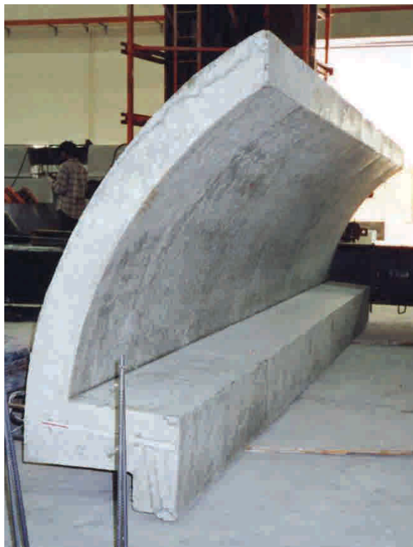
Fig. 1.12 – Vertical casting may be required for curved panels
