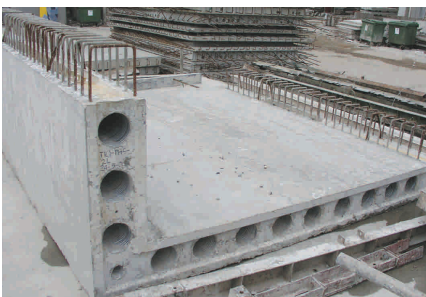
Fig. 1.29 – Precast 'L-shaped' wall panels for shelter construction
