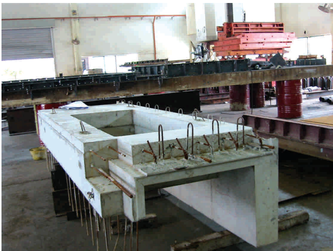
Fig. 6.40 – Bay window integrated with load-bearing vertical elements
