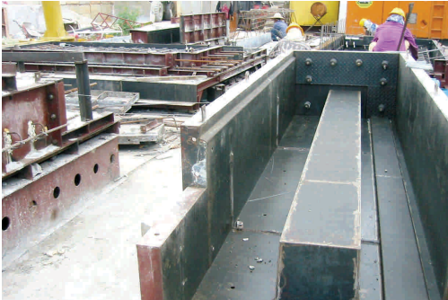
Fig. 6.44 – The fabrication of the precast mould takes into account the blockouts, recesses, groove lines etc. to create the necessary profiles and eliminate “re-work” at site
