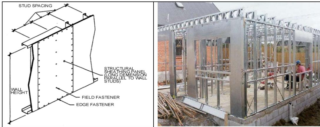
Figure 10.5 Structural Sheathing Fastening Pattern
