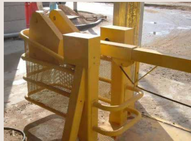
Figure 13: An anti-ramming arm barrier
