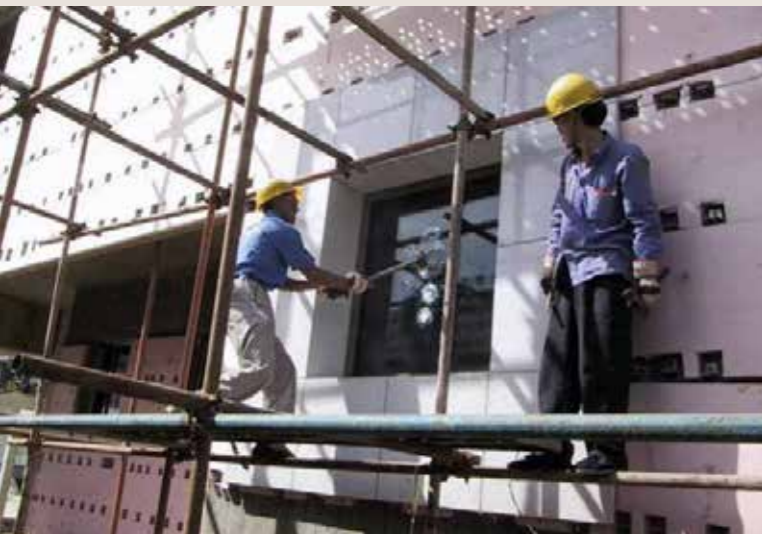
Figure 38: Testing of 15 minutes forced entry resistant window
