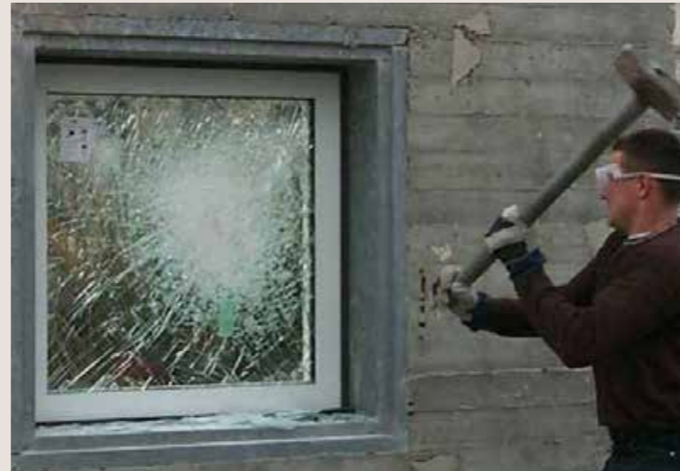
Figure 37: Testing of 15 minutes forced entry resistant window
