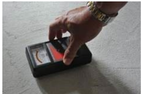
Checking moisture content Figure 4.1.f
