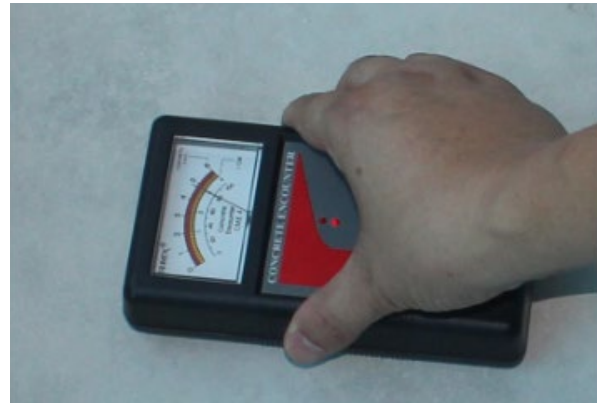
Checking surface moisture content Figure 4.2.2.b
