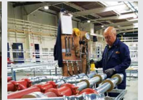
Testing and commissioning of prefabricated MEP Ceiling Module in the factory Photo credits: DSG Modular, Newcastle, England, UK
