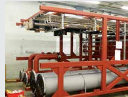
Prefabricated MEP Ceiling Module Photo credits: DSG Modular, Newcastle, England, UK
