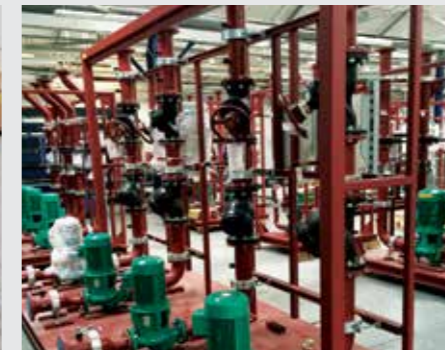
Prefabricated Pump Skid Module Photo credits: DSG Modular, Newcastle, England, UK
