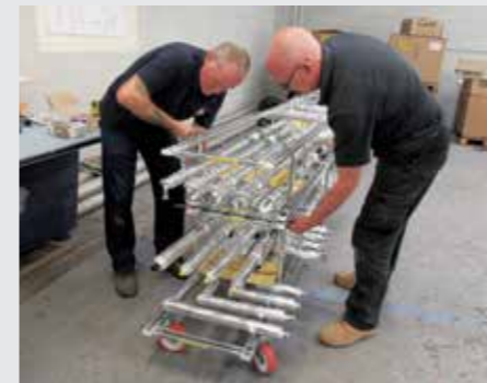
Fabrication of prefabricated MEP ceiling module in the factory Photo credits: DSG Modular, Newcastle, England, UK
